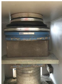
Figure 5.1: Compressive strength test for rubbercrete solid brick
