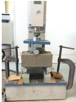
Figure 5.2: Three point test set up for rubbercrete interlocking brick
