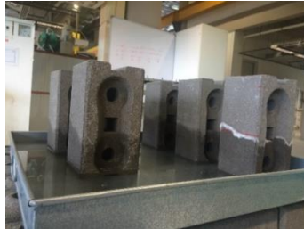
Figure 6.3: RIBs partially immersed in distilled water for efflorescence test
